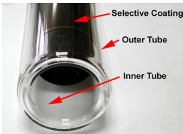
Glass vacuum tubes are the key component of solar water heaters and solar collectors. Each vacuum tube consists of two glass tubes. The outer tube is made of extremely strong transparent borosilicate glass that is able to resist impact from hail up to 25mm in diameter. The inner tube is also made of borosilicate glass, but coated with a special selective coating (Al-N/Al), which features excellent solar heat absorption and minimal heat
