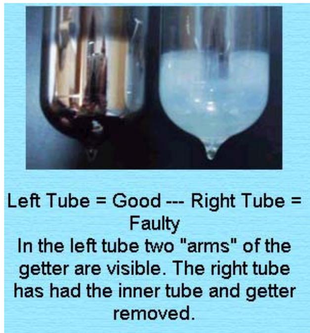
Vacuum tube solar water heater and solar collectors still provide excellent results on cloudy days. This is because the tubes are able to absorb the energy from infrared rays which can pass through clouds. Wind and low temperatures also have less of an effect on the function of evacuated tubes when compared to flat plate solar collectors due to the insulating properties of the vacuum.
